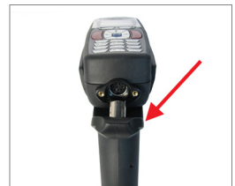
Figure 4 - pull the connector on the handle away from the reader to release the reader
