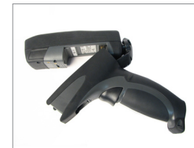
Figure 3 - pull the reader away from the handle
