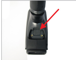
Figure 17 - put the connector into the reader
