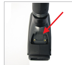
Figure 2 - pull the tab to release the reader from the handle
